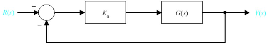
Block diagram of closed-loop system.
