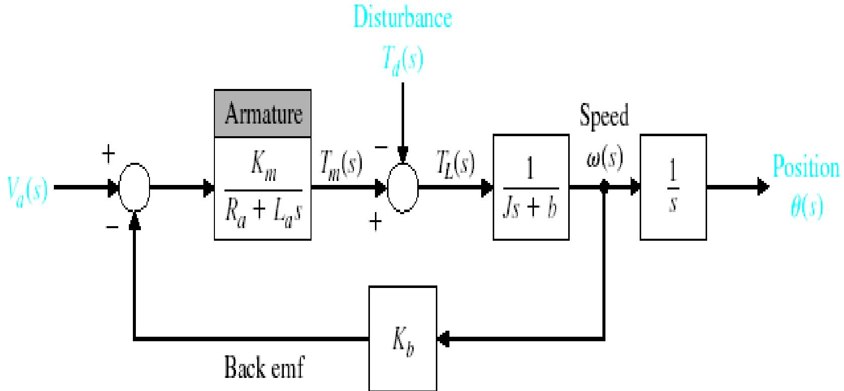
Armature-controlled dc motor.
