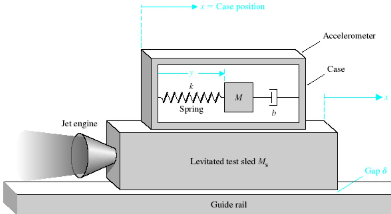
An accelerometer mounted on a jet-engine test sled.
