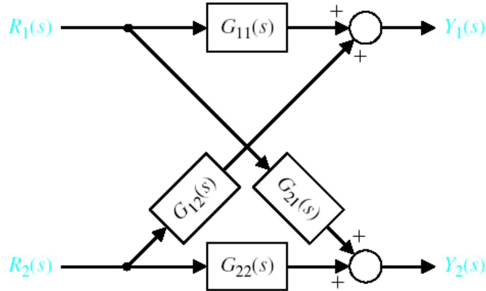
Block diagram of interconnected system.
