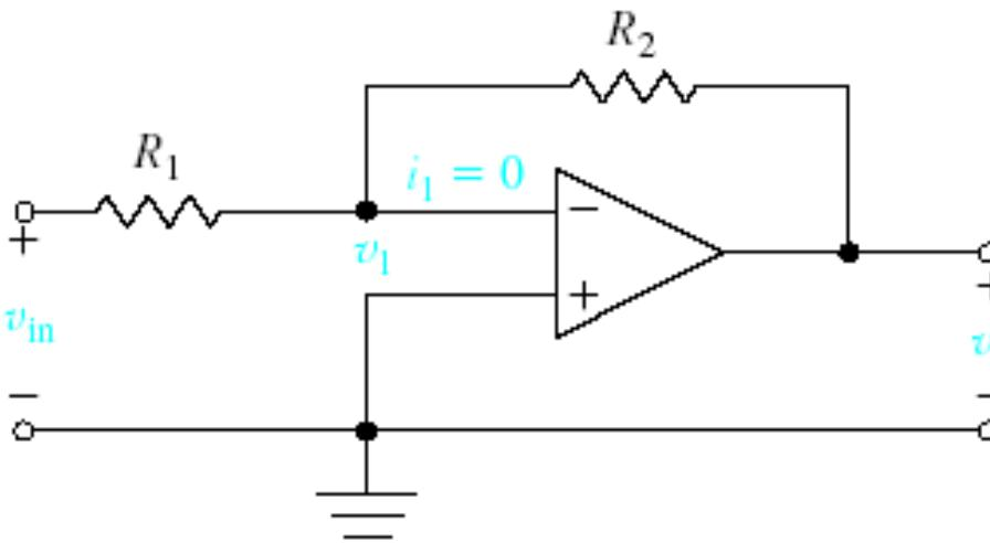
An inverting amplifier operating with ideal conditions.
