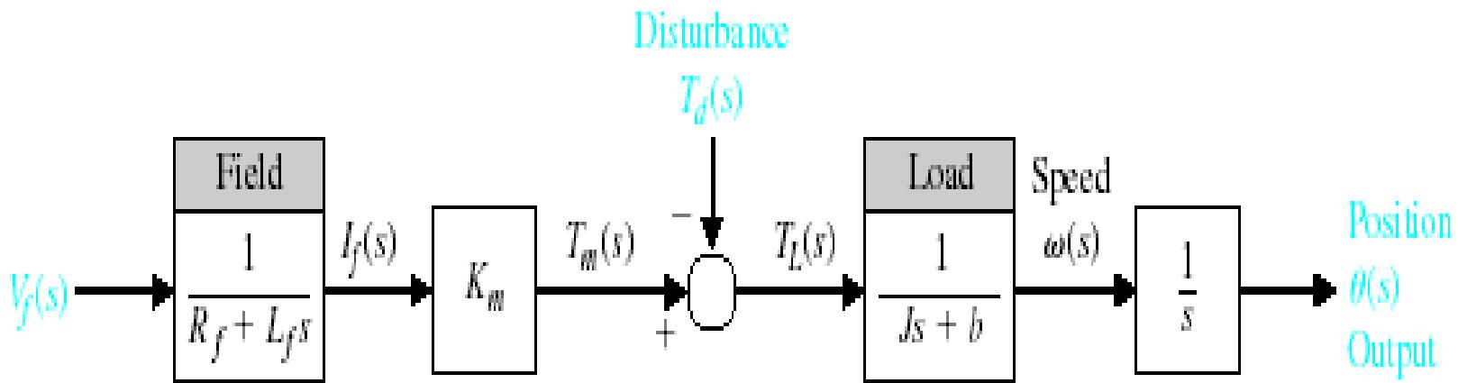
Block diagram model of field-controlled dc motor.
