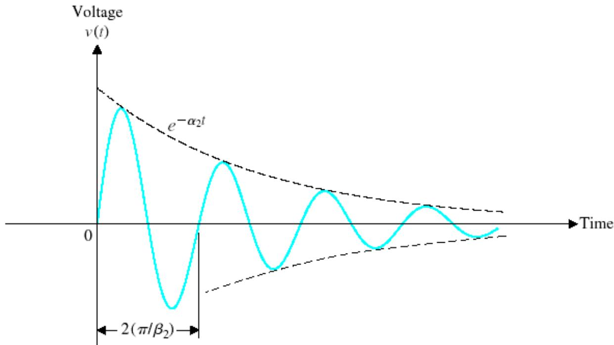
Typical voltage response for underdamped RLC circuit.
