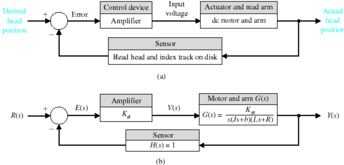
Block diagram model of disk drive read system.
