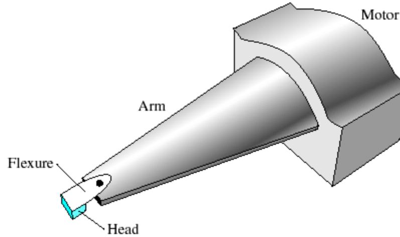
Head mount for reader, showing flexure.
