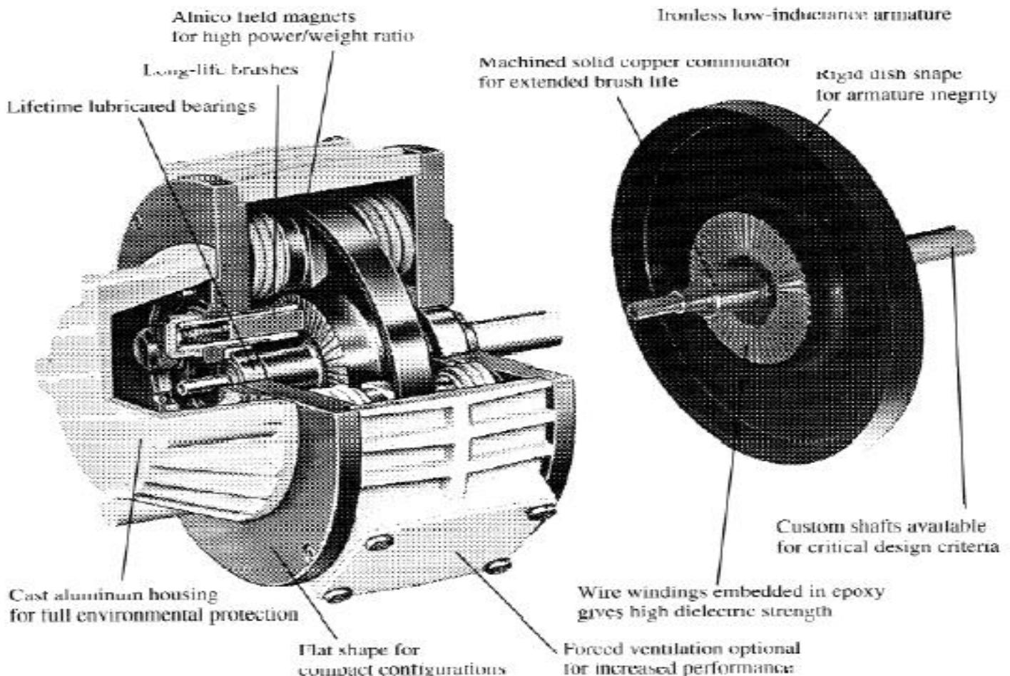
A pancake dc motor with a flat-wound armature and a permanent magnet rotor. These motors are capable of providing high torque with a low rotor inertia. A typical mechanical time constant is in the range of 15 ms. (Courtesy of Mavilor Motors.)
