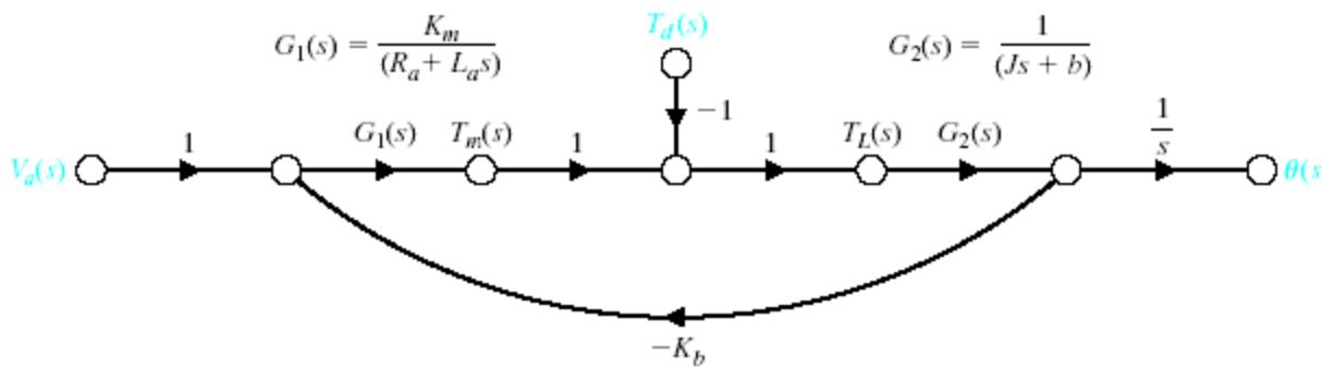
The signal-flow graph of the armature-controlled dc motor.
