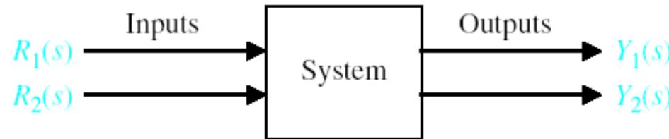
General block representation of two-input, two-output system.
