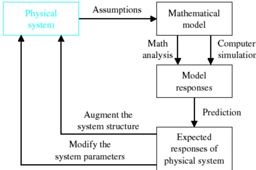
Analysis and design using a system model.
