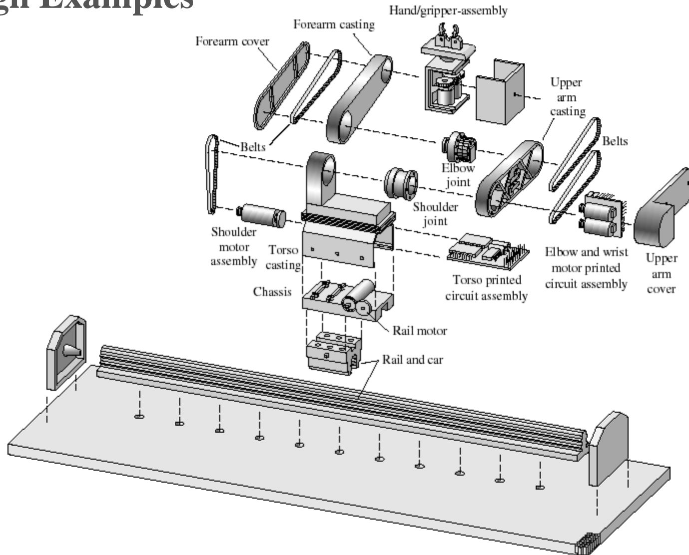
Exploded view of the ORCA robot showing the components [15].
